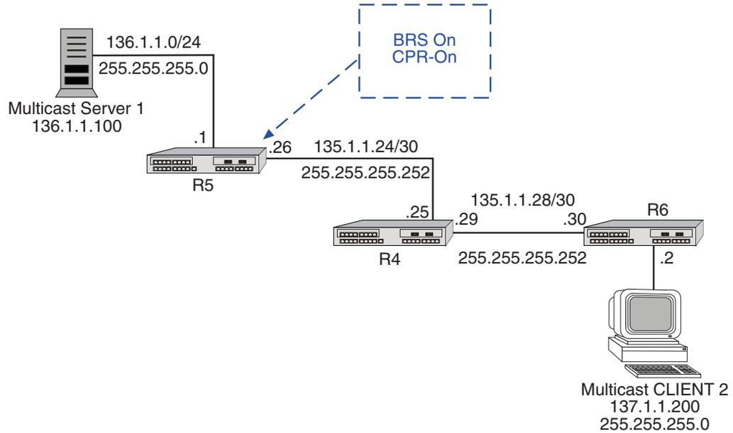
**Figure 34. Using RIPv2, OSPF, and BGP to provide route information for PIM-SM**
