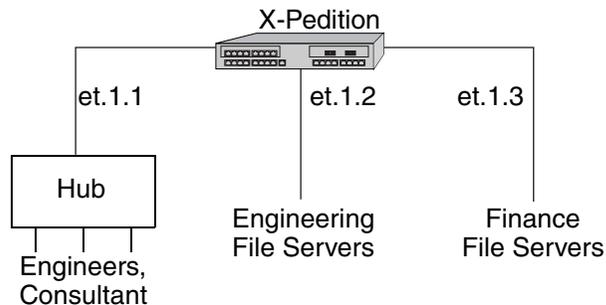
**Figure 40. Source Filter Example**
