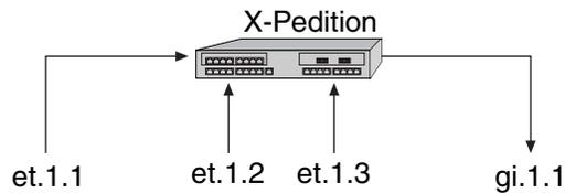
Ports et.1.1, et.1.2 and et.1.3 are being mirrored out gi.1.1
