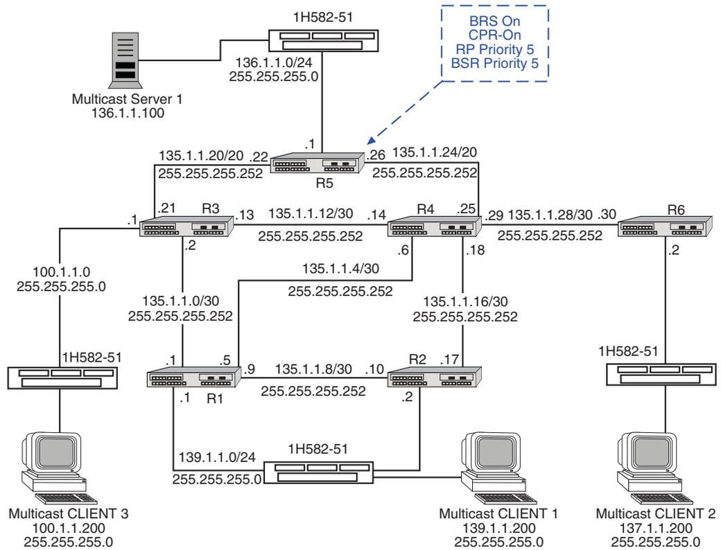
**Figure 35. Configuring the PIM DR, BSR Address, CRP Address, and Static RPs**
