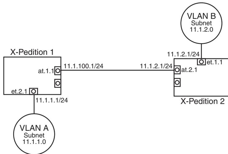
The network shown consists of two X-Pedition routers, VLAN A, and VLAN B. Both routers have an ATM module with two ATM ports. Also both routers contain a 10/100 TX Ethernet module. X-Pedition 1 is connected to VLAN A through Ethernet port et.2.1, while X-Pedition 2 is connected to VLAN B through Ethernet port et.1.1.
