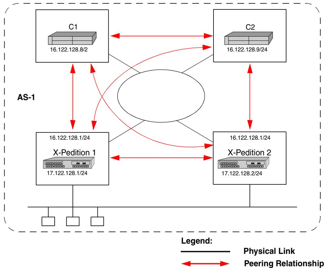
Figure 25. Sample IBGP Configuration (Internal Group Type)
