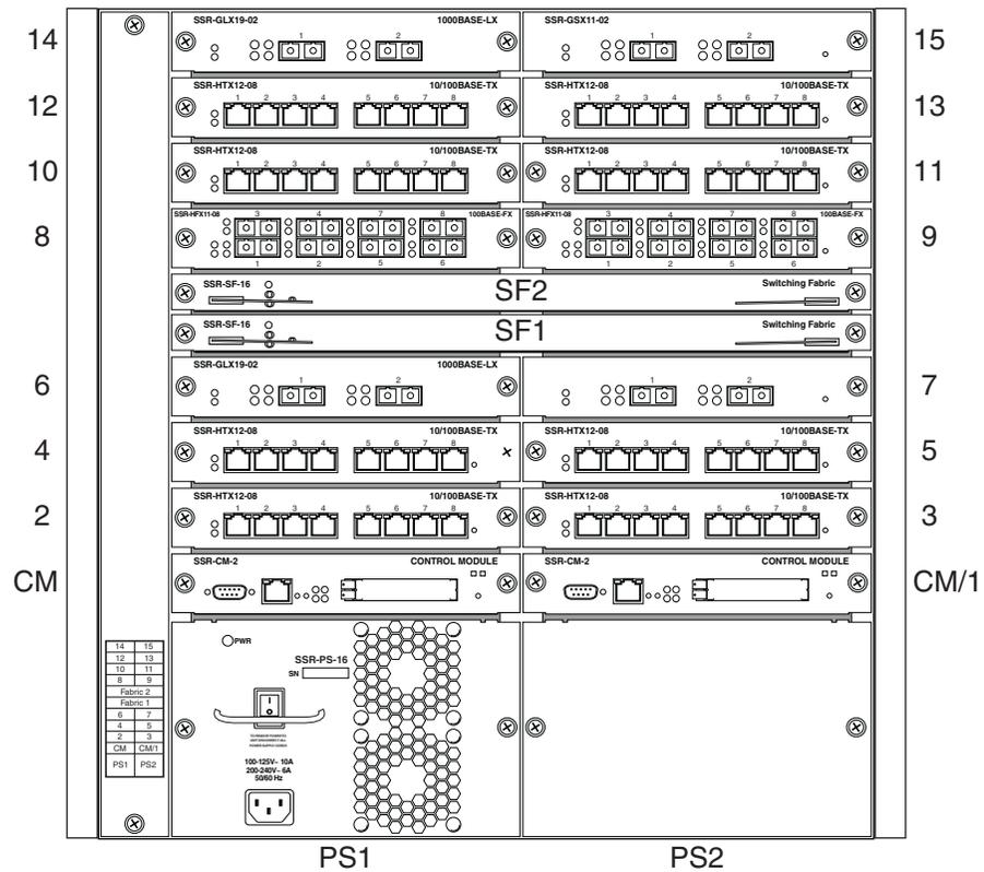
Slot numbers for the vertically arranged line cards of the ER16 are printed just above the slot (Figure 11). ER16 slot 9 can be used for either a second control module or a line card.
