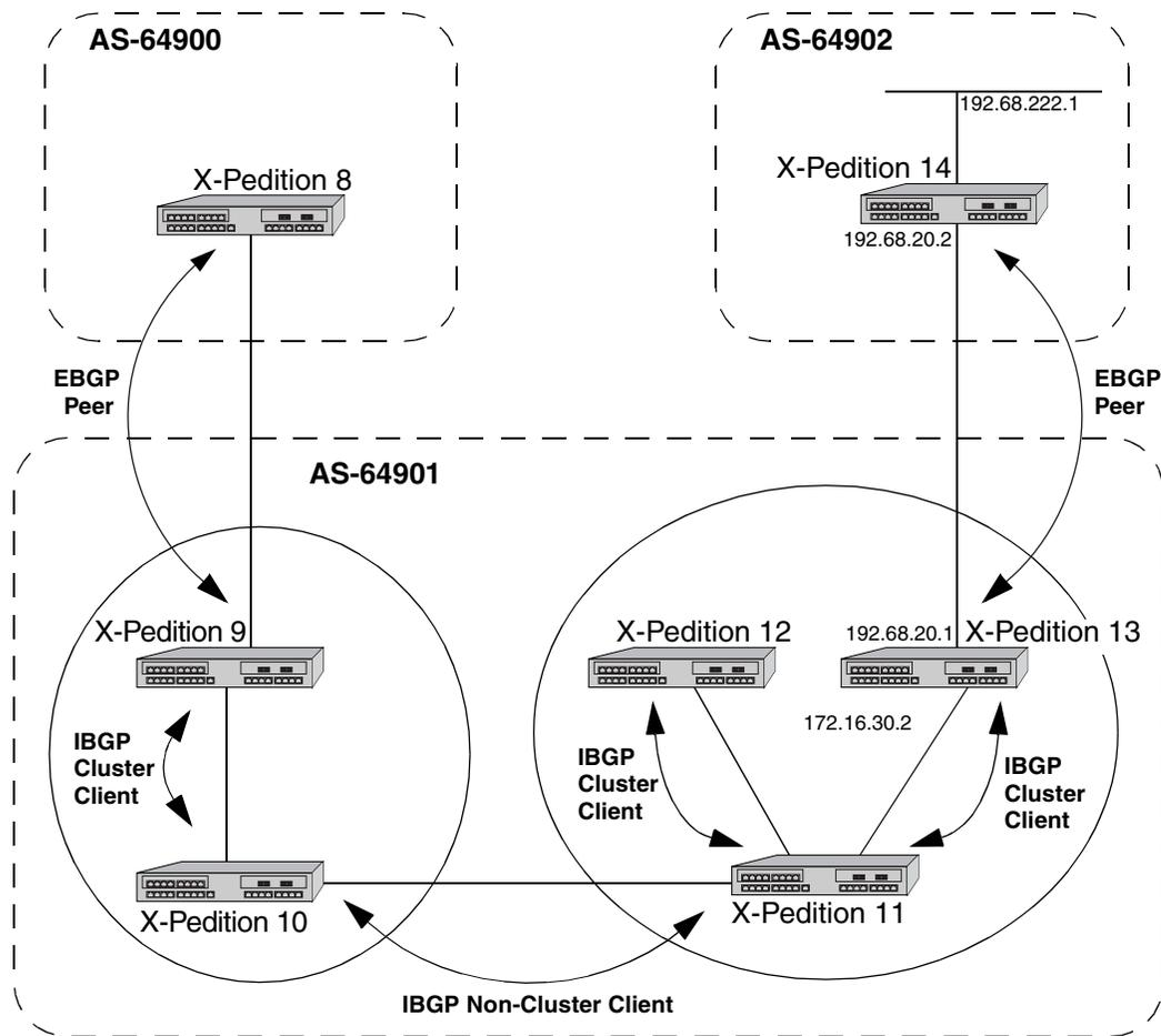
Figure 31. Sample BGP Configuration (Route Reflection)
