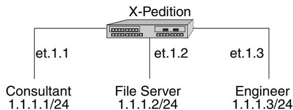
**Figure 41. Sample VLAN for Layer-4 bridging**
