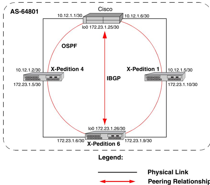
Figure 24. Sample IBGP Configuration (Routing Group Type)
