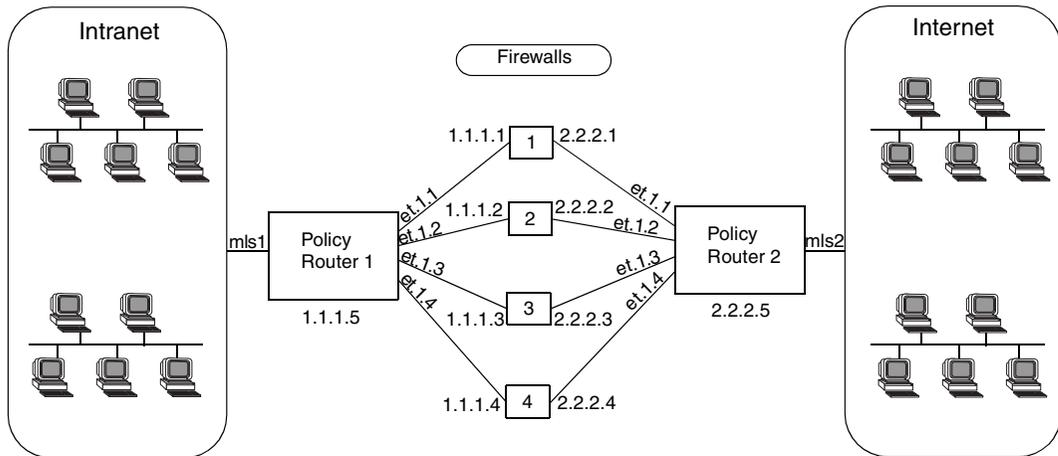
**Figure 39. Selecting Next Hop Gateway from IP Packet Information**
