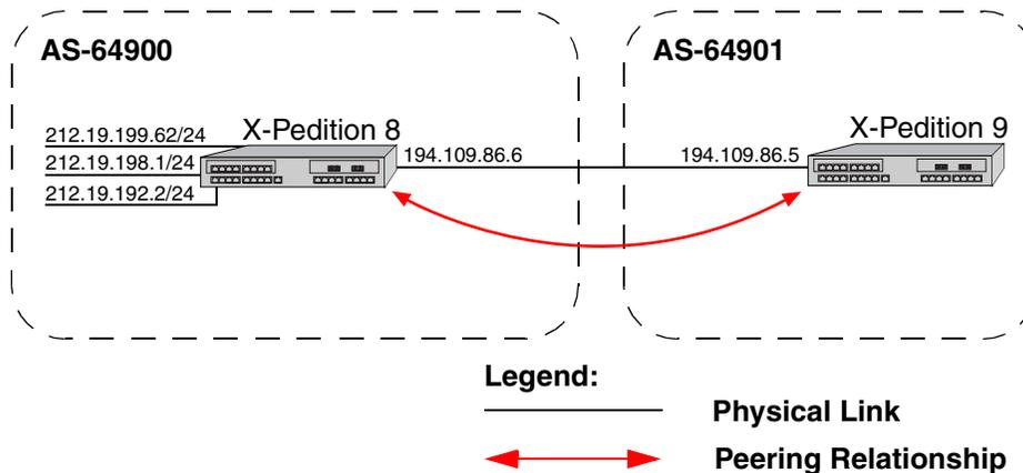
Figure 30. Sample BGP Configuration (Route Aggregation)
